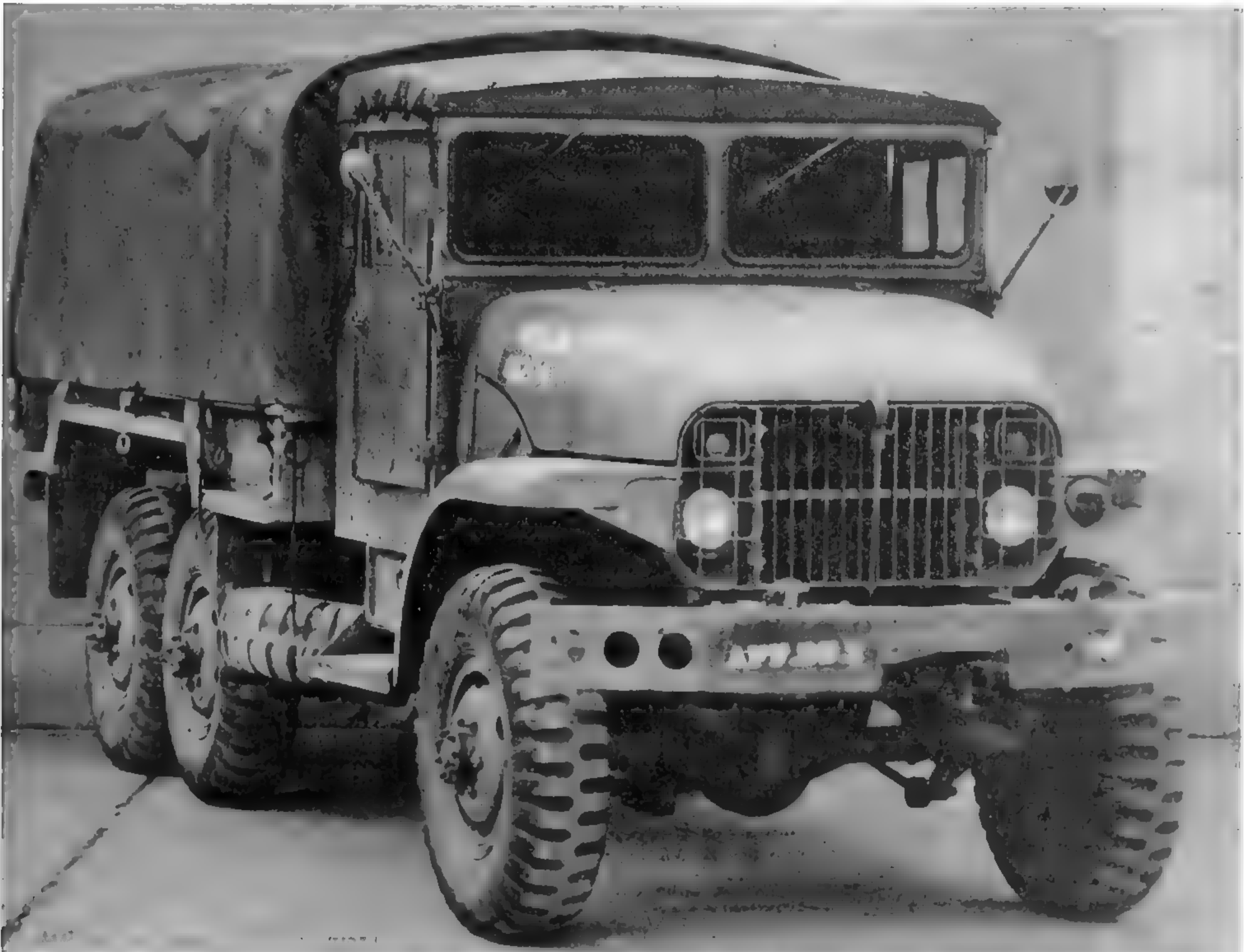
This XM135 received some modifications during testing at Aberdeen Proving Ground. Although the truck's sealed windshield didn't see production, the simple hinged hood prop seen here hanging in the center of the brush guard was adopted. (Photo courtesy of the Patton Museum)
